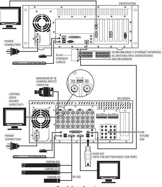
Figure 8. System Connections
